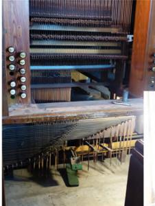
will continue for about 12 weeks. All 745 pipes will be removed from the organ chamber and reshaped as necessary with some of the work being undertaken at the Church and the remainder in the contractor's workshop. The cost is in the order of £11,600
